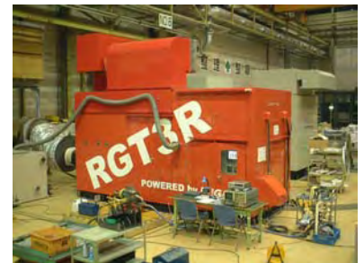
The 300 kW Niigata RGT3R Recuprated Cycle Gas Turbine, using a Dry Low Emission Combustor. Courtesy of Niigata Power. Co.
